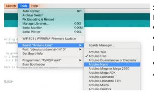
Start up your computer, attach the Grains'Arduino Nano board to your computer using a data usb cable. Open the Arduino IDE program. You will download the code later, first you have to select the right board, processor and COM port.
