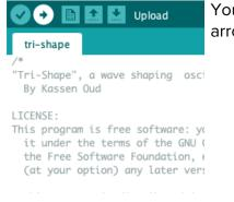
You can upload the code to the Arduino Nano board by clicking on the arrow pointing right, in the dark green bar on the upper left of the IDE.
